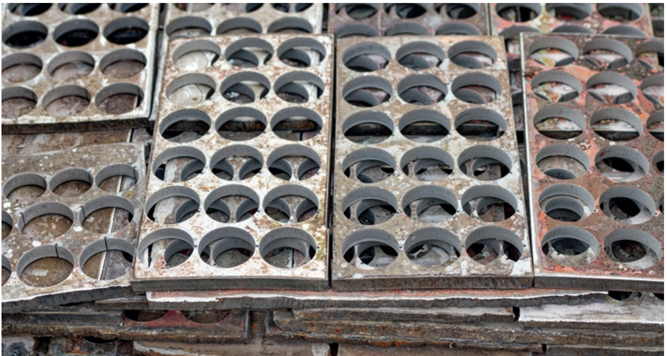
Optimal material utilisation thanks to CAD-controlled water jet cutting system. The leftover pieces are also recycled.
