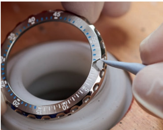
The illuminated triangle of the rotating bezel is set and bonded by hand.
