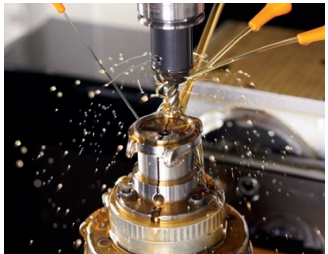
An almost finished case middle on an automatic processing machine at SUG.
