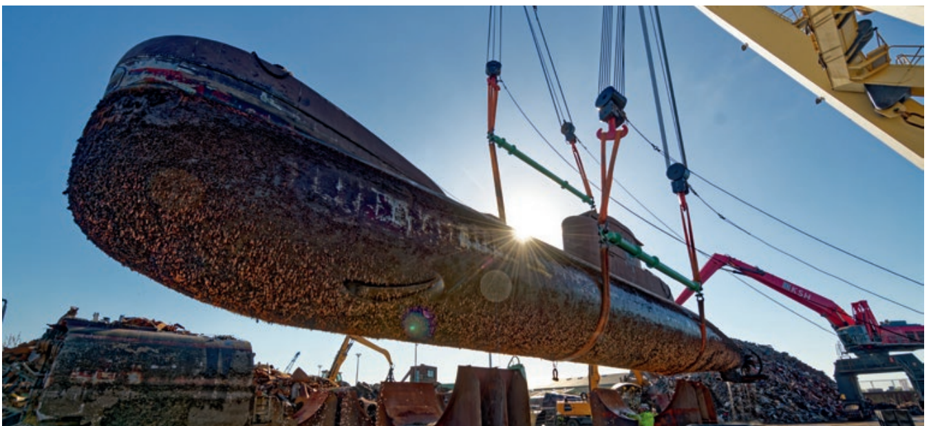
9.00 a.m.: The floating crane lowers the U 15 - which weighs some 450 tonnes - into the so-called cradle. Here, the submarine is kept stable until the hull is dismantled.
